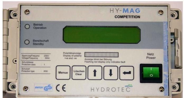
The Competition control box can be programmed to operate in a time controlled or continuous mode, although we strongly advise that the unit should operate in a continuous mode.
